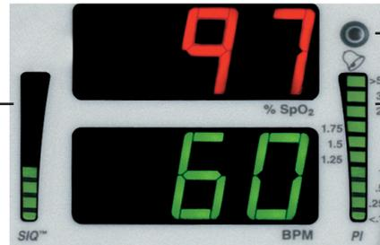
The Alarm Status Indicator flashes when an alarm condition is present.
